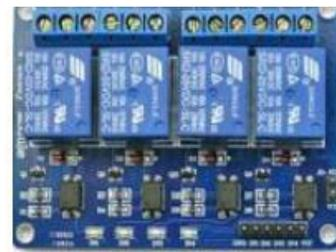
Gambar 2.5 Relay 4 channel
